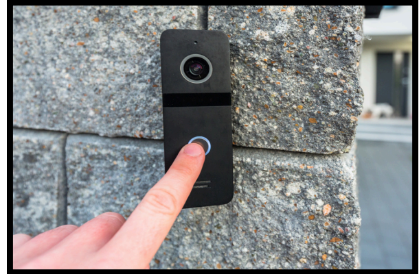
2. Camera is activated when it detects motion or the doorbell is pressed
